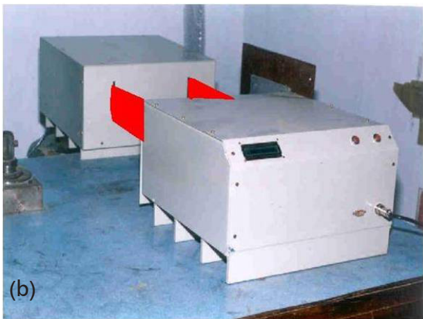
Fig. 5: a. Block Diagram, b. Photograph, of the Laser velocity meter
