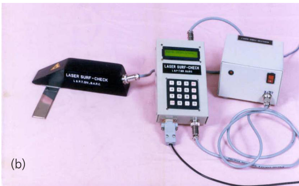
Fig. 3: a. Schematic Diagram of Laser based roughness measuring instrument, b. Photograph of Laser Surf-check
