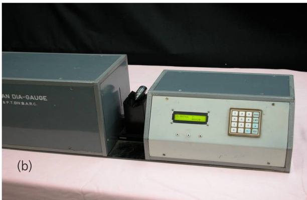
Fig. 2: a. Schematic of Laser based diameter measurement, b. Photograph of Lascan Dia-Gauge
