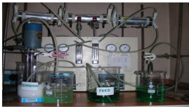
Fig. 2: Experimental set up of 3 small HF contactors in series operating in once through mode; Flow rate: 12LPH; Feed: U raffinate; dispersion: aq/org 1:1, aq (1 M NaHCO 3 ), org (30 % v/v TBP in Dodecane)
