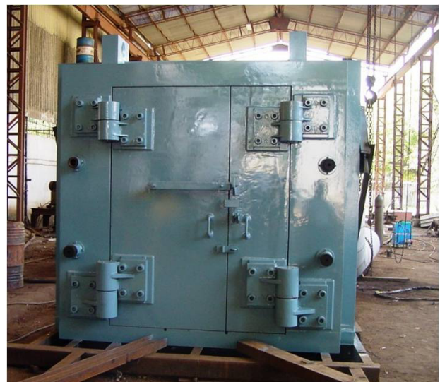
Fig. 4: Personal Access Door of ACHF, Kota at Fabricator's Shop
