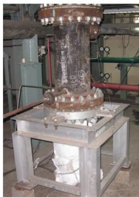
(a) Melt coolability under top flooding
