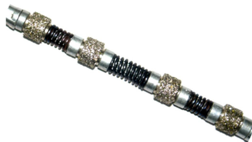
Fig. 9: Electroplated diamond wire used during wire sawing demonstration
