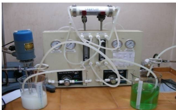
Fig. 1: Single hollow fiber contactor set up operating in recirculation mode; Flow rate: 12LPH; Feed: U raffinate; dispersion: aq/org 1:1, aq (1 M NaHCO 3 ), org (30 % v/v TBP in Dodecane)
