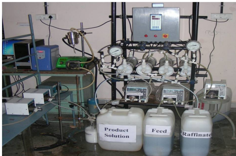
Fig. 5: Bench scale set up: Four large HF modules in series Feed: U raffinate; dispersion: aq/org 1:1, aq (1 M NaHCO 3 ), org (30 % v/v TBP in Dodecane); flow rate: 60LPH
