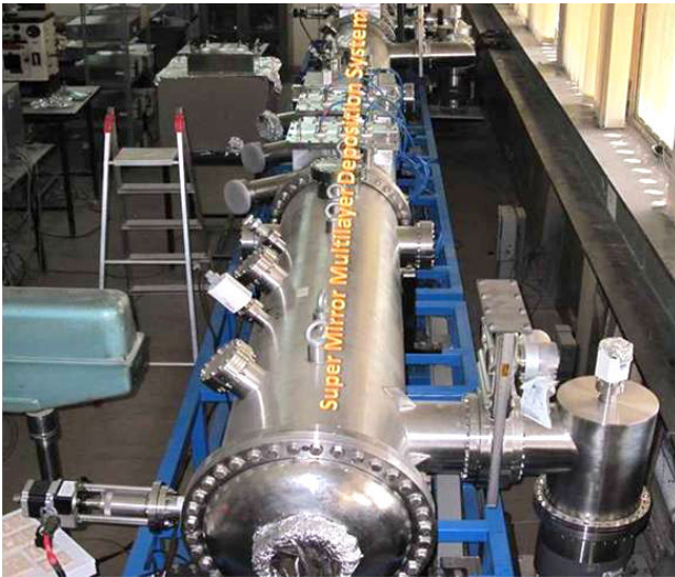
Fig.11: An indigenously developed magnetron sputtering system for super mirror developments at A&MPD
